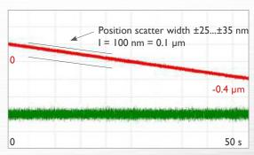
Red line: Path 0... -0.4 µm in 50 seconds Green line: Speed (0.5 µm/min)
